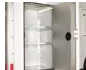
Exterior compartments now feature integrated shelf brackets with more locations – and aluminum-lined doors include strong, automotive door seals and stainless steel hinges.
