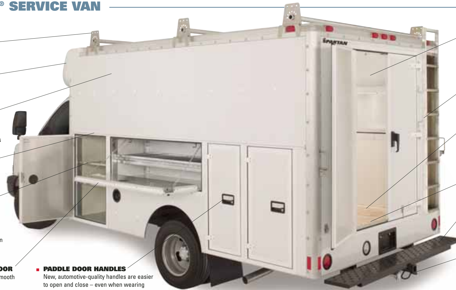
Body shown with optional ladder rack, rear access ladder, fixed interior shelves, Master Lock® system, and receiver hitch tube.
