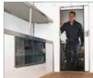
Spartan's Top Hat cab with full-height cab-access door lets you stand upright to move between the cab and cargo area.
