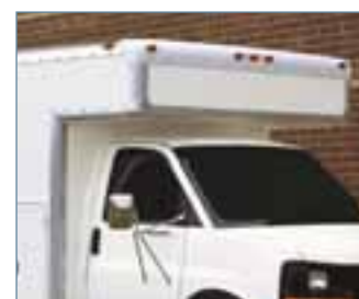
Opt for the cab-over storage attic in lieu of the wind faring, and you'll have extra room for even more cargo.
