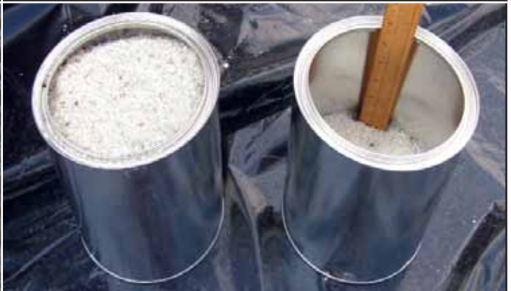
Rock Salt quantity shown before and after being refined in the Salt Slurry Generator.
