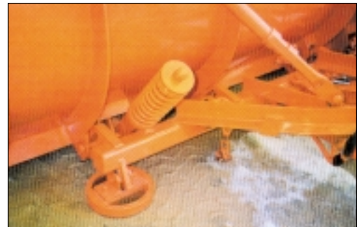
Two adjustable Compression Springs are conveniently located with (4) HD slotted trip lugs to provide safe trip action.
