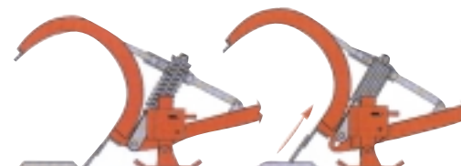
Slotted Trip Moldboard shown tripping over obstacles.
