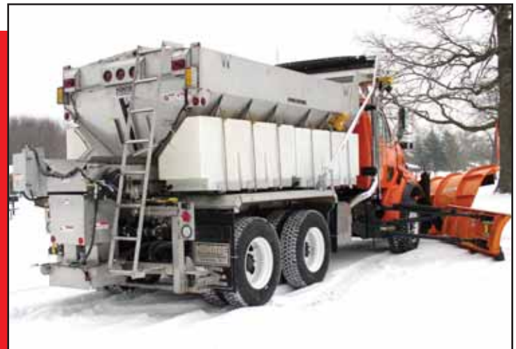
Chassis mount, 14' v-box, 720 gallons of liquid, prewet, custom light package & 3-lane anti-ice corrosion-resistant stainless fenders, top grates, and ladder. ▶
