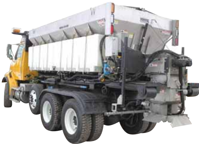
Chassis mount, 14' v-box, 720 gallons of liquid, prewet, custom light package & 3-lane anti-ice corrosion-resistant stainless fenders, top grates, and ladder. ▶
