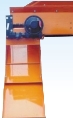
Berm Chute in operating position
