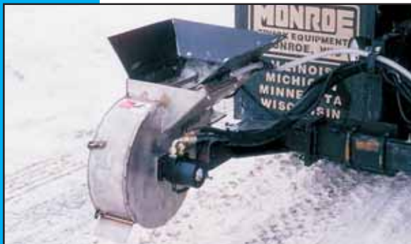
Shown with standard 12" x 14" opening with three flexible bolt-on flares that help divert granular material into housing.
