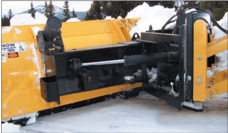
The new and improved LGP plow shown with outboard cylinder setup, 2" cylinder pins and cylinder ears.
