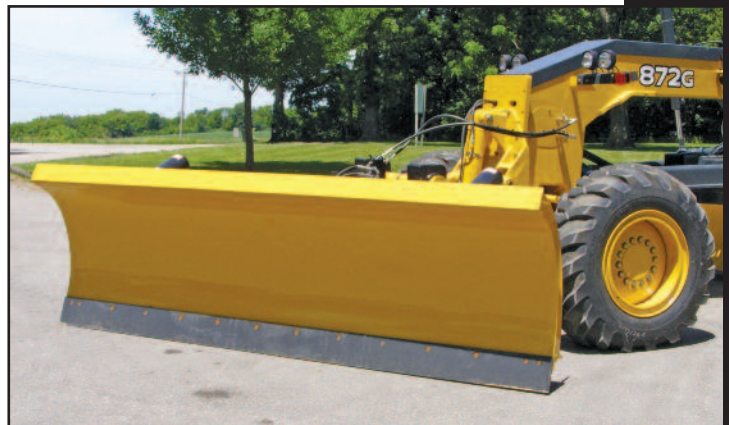
Maximum Single-Pass Coverage--The standard 12' LGP plow produces a 10'2" clearing path when fully angled, which is ideal for clearing the front steering wheels & feeding the snow load onto the wing behind it.
