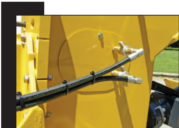
Monroe typically uses "couple-under-pressure" wing-type fittings to speed implement attachment and detachment from the loader or motorgrader
