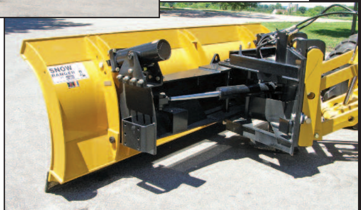
A variety of female coupler hook options are available, such as these B-Type hooks, which mate up to Deere's optional front lift group.
