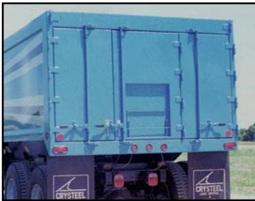
Standard 3-door rear gate with center grain chute.
