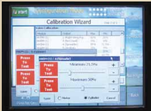
Valve Calibration Wizard. Calibrate on screen step by step.
