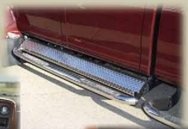
Step Tubes with Polished Stainless Steel Kick Plate
